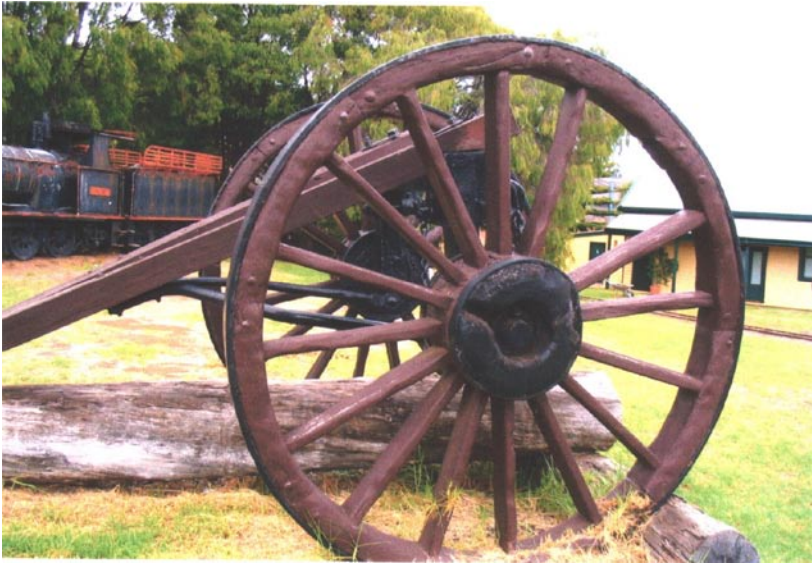
Figure 5. A whim, used for hauling large logs in the karri forest.
